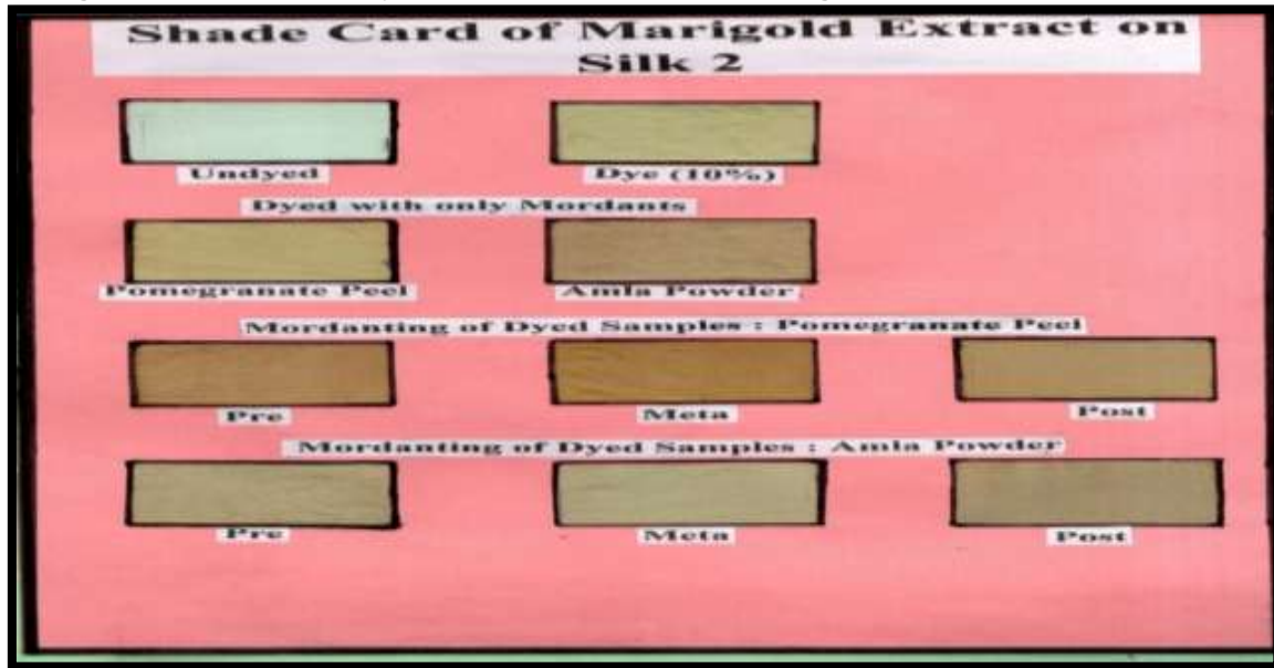
Figure 3: Shade card of Dyed Fabric Samples of Silk with Tagetes Erecta and Natural Mordants
